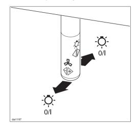
To turn the light on or off, press the joystick either once backwards or once forwards.
